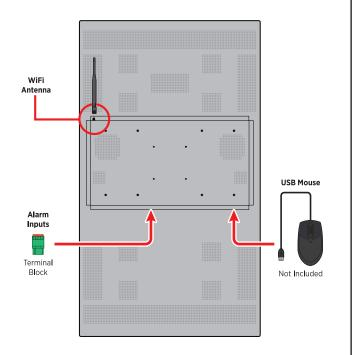
If desired, connect alarm input connections using the included 4-Pin terminal block.
