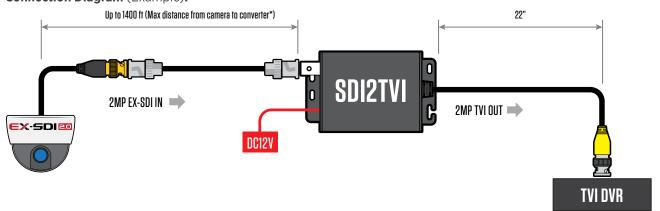
\*Distances will vary depending on coax cable type & integrity. Cable splices, couplers and severe kinks will reduce the overall possible distance.
