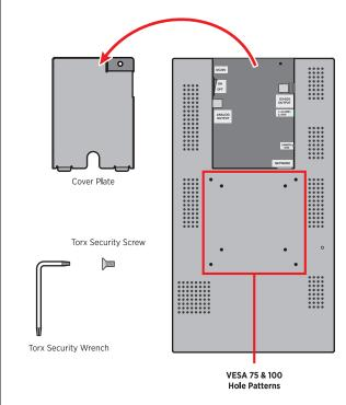
\*Replace Cover and Security Screw when setup is complete.
