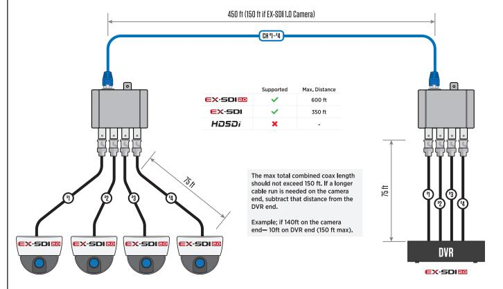
\*Distances shown based on new CAT5e ethernet cable & new RG59/U (20AWG) coaxial cable.
