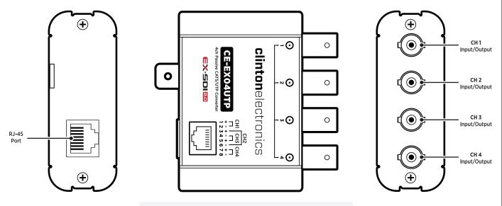
Connections are Non-directional: can be used as an Input or an Output
