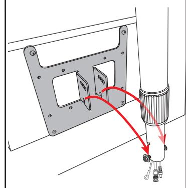
\*TIP- Hang the monitor with the back of the monitor facing you. This way you can easily see the plate aligning to the support bolt, as well as insert the top bolt to secure it in place.
