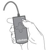
**[EXIT]** Exits the menu, changes are temporarily held- changes will be lost when camera is power cycled (On>Off>On).
