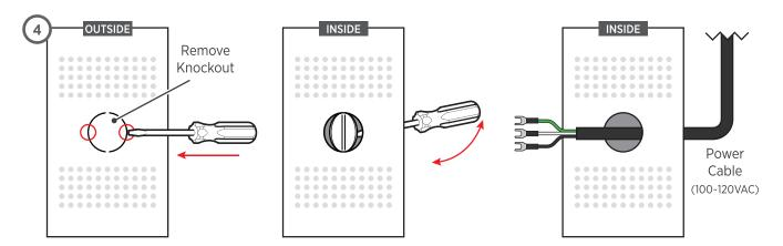
**4.** Remove a knockout on the bottom half of the enclosure. (It may be easier to remove the knockout with the enclosure off the wall) To remove a knockout; push/strike inward with a flathead screwdriver or chisel on either side of the knockout. After the knockout is loose, pry the screwdriver and knockout from side to side to remove from the enclosure. Once the knockout is removed from the bottom half of the enclosure, insert the Power Cable into the enclosure.
