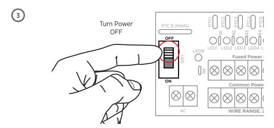
3. Slide switch on Power Supply PD (Power Distribution) board to OFF position.
