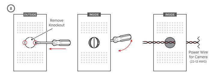
8. Remove separate knockout(s) for the low voltage camera wiring. It is recommended to use a knockout on the top half of the enclosure. DO NOT use the same knockout opening as the main power source. Once the knockout(s) are removed from the top half of the enclosure, insert the Camera Power Wires into the enclosure. (Camera Power Wires Not Included).
