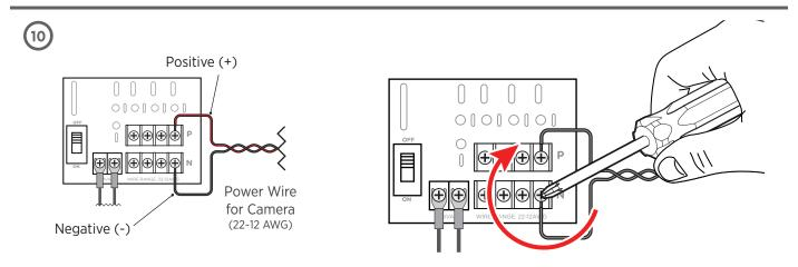
**10.** Connect CCTV cameras (or other external loads) to appropriate terminals, carefully observing polarity. Tighten terminal connections with Phillips head screwdriver.
