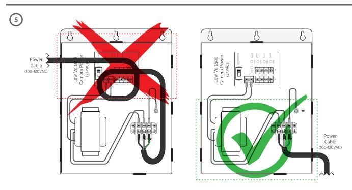
**5.** Route the Power Cable through the hole made from removing the knockout on the bottom half of the enclosure. Ensure that the Power Cable maintains a distance of at least 1/4" from the low voltage DC camera power.
