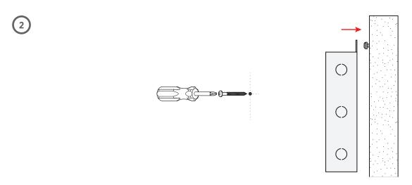
2. Install two upper fasteners (sufficient length 1/8" bolts or screws, not included) in the wall with the screw heads protruding. Place the enclosure's upper keyholes over the two upper screws, level and secure. Mark the position of the lower two hole(s). Remove the enclosure. Drill the lower hole(s). Place the enclosure's upper keyholes over the two upper screws. Install the lower screw(s) and make sure to tighten all screws. Secure enclosure to earth ground.
