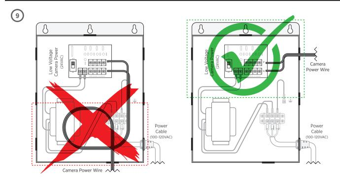
**9.** Route the Camera Power Wires into the hole made from removing the knockout on the top half of the enclosure. Ensure that the low voltage AC camera power maintains a distance of at least 1/4" from the main AC power.
