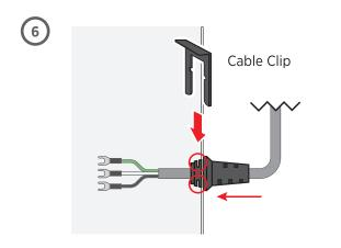
**6.** Secure the Power Cable to the enclosure with the supplied clip. Push boot on cable firmly against the enclosure and slide the clip into the notches on the boot from inside of the enclosure.
