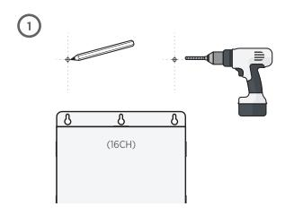
Mark and pre-drill holes on the wall where enclosure is to be mounted. Choose a vertical surface (wall) strong enough to support the full weight of the assembly. Select a mounting location in an area without excessive moisture; for indoor installation only and in a secured area.
