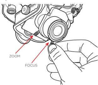
After zoom / focus adjustments have been made, tighten the adjustment levers to lock the adjustments.
