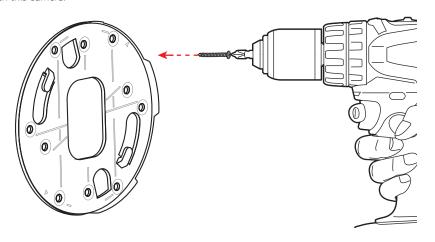
NOTE: It is recommend to use drywall anchors if mounting to drywall. Drywall anchors not included.
