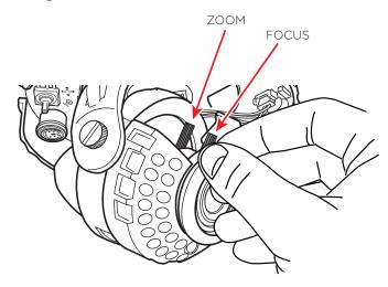
After zoom / focus adjustments have been made, tighten the adjustment levers to lock the adjustments.
