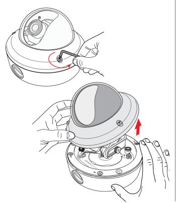
**b** Locate and remove the 4 Phillips head screws that hold the inner case onto the camera base. Remove the inner camera case from the camera base as shown below.
