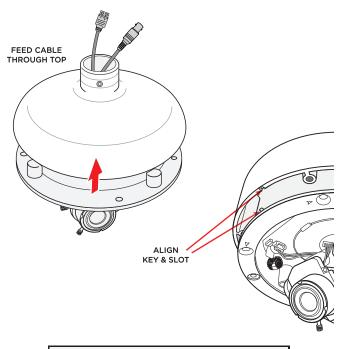
IF KEY & SLOT ARE NOT ALIGNED PROPERLY THE WEATHER RESISTANT SEAL WILL BE COMPRISED. ALLOWING WATER TO LEAK INTO THE CAMERA.
