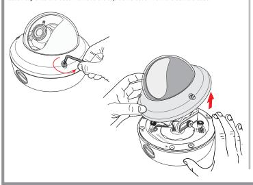
D. Remove the four Phillips head screws that hold the inner case onto the camera base, then remove the inner camera assembly from the camera base.
