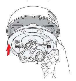
**b**<sub>•</sub> Align the key on the lip of the inner camera assembly with the slot on the camera base when reassembling. If these are not aligned properly the weather resistant seal will be comprised, allowing water to leak into the camera.
