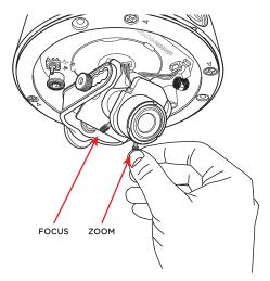
After adjustments have been made make sure to tighten the adjustment levers to lock the adjustments into place.
