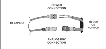
To ensure quality operation, verify proper BNC and power termination; along with proper voltage at camera.
