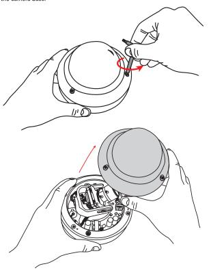
$f b_*$  Locate and remove the 4 Phillips head screws that hold the inner case onto the camera base. Remove the inner camera case from the camera base as shown below.
