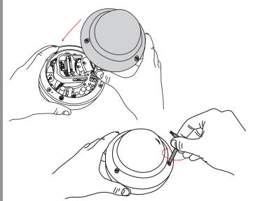
**b**. Make sure each screw is tight to ensure superior weather resistance.
