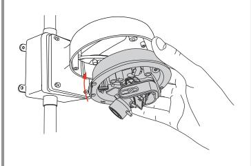
**b.** Align the key on the lip of the inner case with the slot on the wall bracket when reassembling. If these are not aligned properly the weather proof seal will be comprised, allowing water to leak into the camera.
