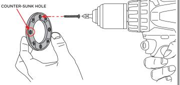
Make sure the gasket side of the mounting bracket is not facing out. If installed this way you will be unable to affix the camera to the bracket.
