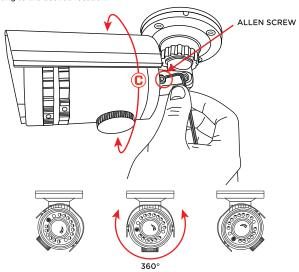
After adjustments have been made make sure to tighten the collar and/or Allen screws to lock the adjustments into place.
