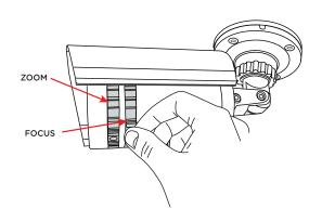
If the adjusting collars do not turn easily it may be necessary to first loosen the screw located under the black button cap. (Use a flat head screwdriver to pry the cap off). Make sure to re-tighten the screw so the zoom/focus adjustments made will not fall out of adjustment.
