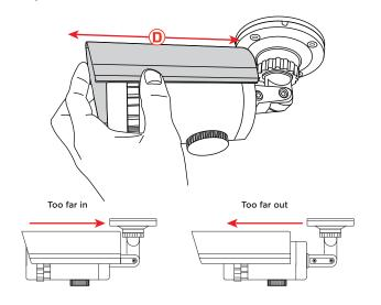
Positioning the sun-shield too far forward could result in a barrel effect when viewing the image, too far to back will not provide protection of the lens from sun light or weather.
