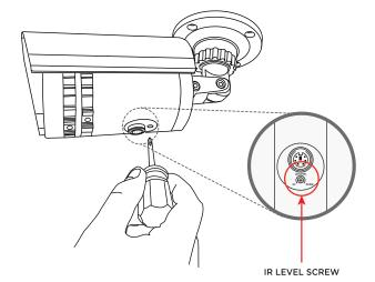
After adjustments have been made make sure to replace the cap to ensure superior
