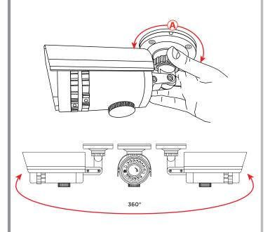
$f b_*$  Lens angle can be adjusted by loosening the appropriate Allen screw, then adjusting to the desired location.
