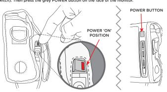
DC12V. Push the grey POWER button on the face of the monitor.
