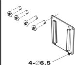
Secure wall mount plate firmly to the wall with four expansion screws (not supplied ).
