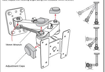
Replace base plate covers and adjustment caps when finished making adjustments
