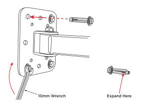
If the bolt assembly does not start to expand, remove it and gently pry the expansion sleeve open to initiate expansion in the hole.
