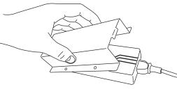
Attach the power supply to the mounting surface with 4 screws (not included).
