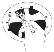
Align the tab with the slot when reassembling.
