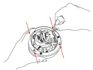
Remove the camera assembly from the camera base as shown below. Set this base aside. You will not need this base when using the Recess Mount.
