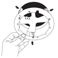
With a Phillips head screwdriver, rotate the three screws clockwise to flip the tension wings out until they firmly grip the mounting material. **NOTE:** When mounting, make sure the mounting surface does not block the three perimeter holes shown below. These holes must be clear in order to accept the VX case in the next steps.
