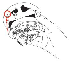
Replace the four screws that hold the camera assembly to the base. Note: Arrowheads indicate screw location.
