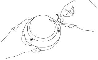
Locate and remove the 4 Phillips head screws that hold the inner case onto the camera base. Note: Arrowheads indicate screw location.
