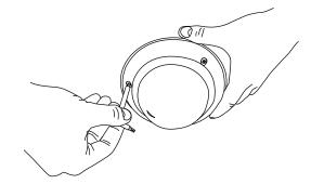
**NOTE:** Due to the replacement of the bottom case, a 1/16" gap between the VXRM and the VX camera dome will result. This will not affect the IP68 weather rating of the VX series camera.
