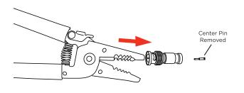
$\mathbf{6}_{\text{\tiny{I}}}$  Insert the center conductor from the cable into the center pin from the connector.
