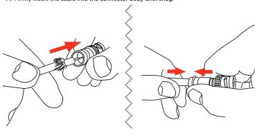
$f B_{\scriptscriptstyle \parallel}$  Insert the cable with the connector into the BNC compression pliers as shown. The tip of the BNC connector should rest on the circular stop of the compression pliers. Swing the cable latch closed at the cable end to secure the cable. Firmly squeeze the handles of the BNC compression pliers all the way closed and then release. Your BNC connection is now complete!
