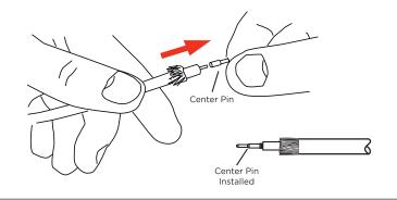
7. Firmly insert the cable into the connector body until snug.
