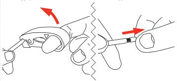
$oldsymbol{4}_{ t s}$  Fold back the copper strands onto the outer shell of the cable. The approximate lengths are shown in the diagram below. Make sure that all of the copper braid is folded back completely and not touching the dielectric or center conductor.
