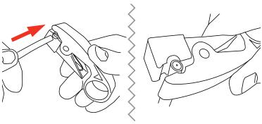
$oldsymbol{\exists}_{oldsymbol{i}}$  Rotate the coax stripper one complete rotation around the cable. Then pull the coax stripper from the cable. If the outer cable insulation segment did not fall off when using the coax stripper, remove this section to reveal the braided copper strands.
