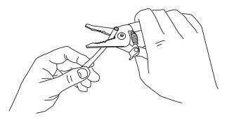
$\mathbf{2}_{\scriptscriptstyle{\mathrm{II}}}$  Insert the cable end into the coax stripper from the left side of the tool as shown. The cable end should be flush with the side of the tool, and resting in the cable guide teeth.
